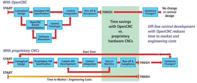
OpenCNC software cuts design cycles by enabling concurrent, non-linear design development.
